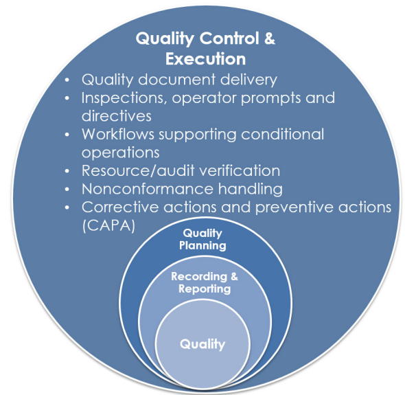
Figure 4. Quality Control and Execution Activities
